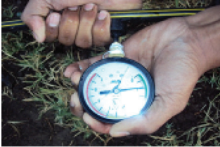
Measuring the pressure by pressure gauge
