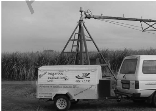
FIGURE 4 "Mobile unit", Mobile irrigation laboratory of ARC-Institute for Agricultural Engineering, South Africa.
