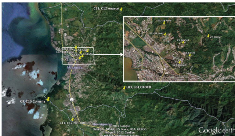
FIGURE 12.13 Detailed rain gauges network.
