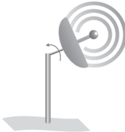
FIGURE 12.11 Range Height Indicator (RHI).
