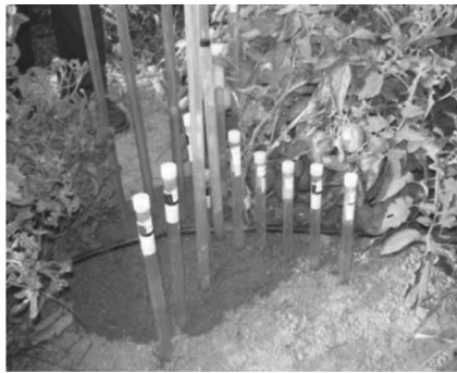
FIGURE 5.2 Measurement of wetted front advance: visual and tensiometric (sensors).
