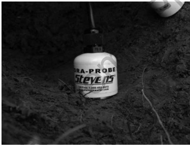
FIGURE 7 Installation of a Stevens Hydra Probe into native soil at a SNOTEL site [2].
