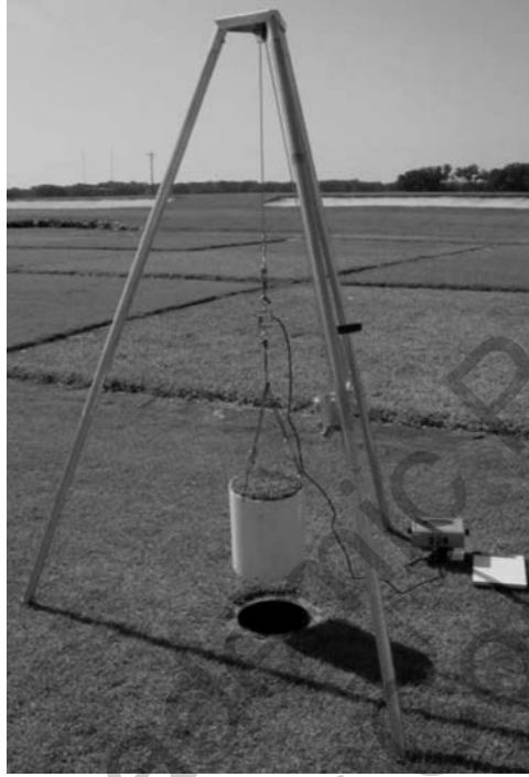
FIGURE 2 Photograph of tripod placement, hoist, load cell, harness, lysimeter, and output display.
