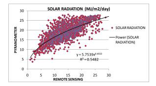
Figure 1. Comparison of solar radiation obtained from pyranometers at six locations in Puerto Rico and satellite remote sensing.
