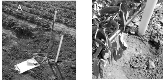
**Figure 4.2.** Soil physical parameters measured in field. **A.** Field capacity test, at two soil depths: 0-20 cm and 20-40 cm. **B.** Undisturbed core sample collection.
