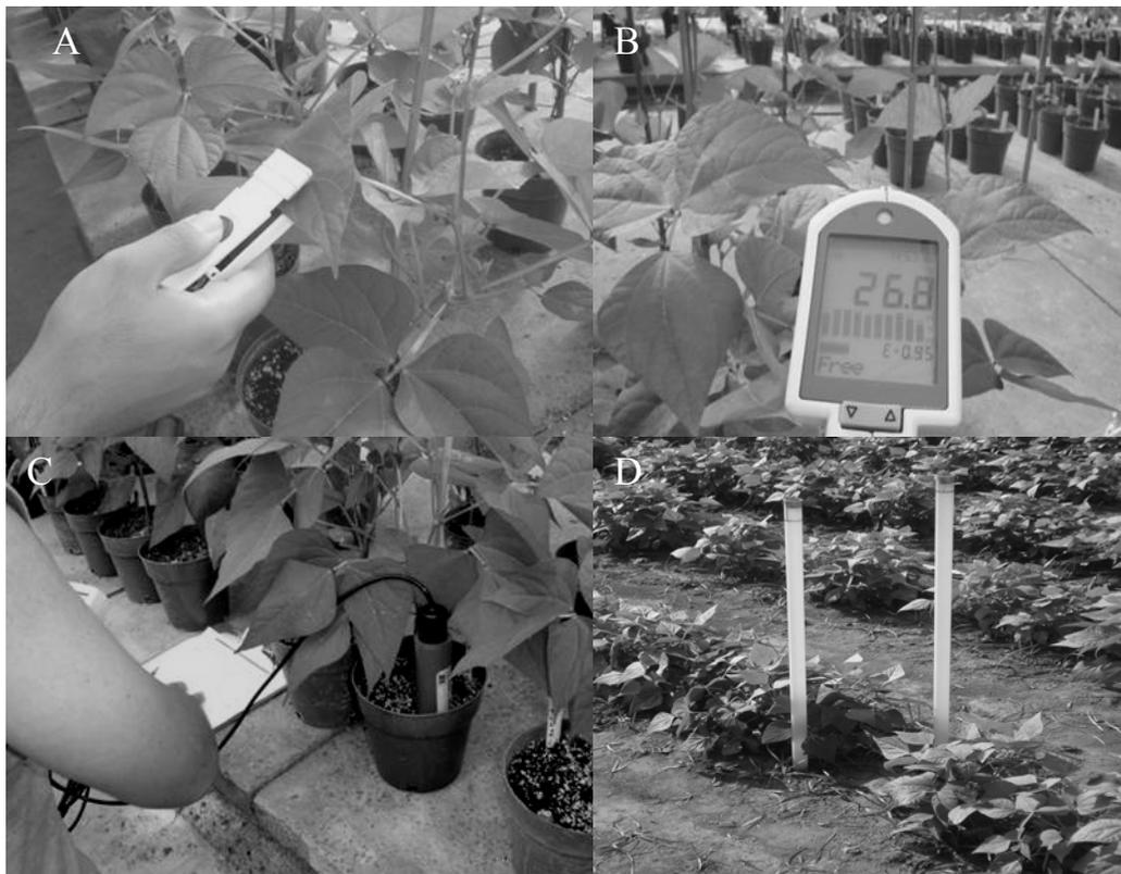
**Figure 3.1.** Equipment used in the greenhouse and field studies: **A.** Leaf porometer; **B.** Infrared leaf temperature sensor; **C.** Volumetric moisture sensor in greenhouse and **D** in field.
