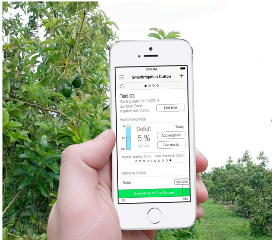
Figure 9: Example irrigation application. In this case, the “smartirrigation cotton” application, to be updated for avocados, with added SM and crop stress/ESI information from ALEXI and GriddSAT, such that growers can have added information so to make more intelligent irrigation decisions, and how to optimize fertilizer applications.
