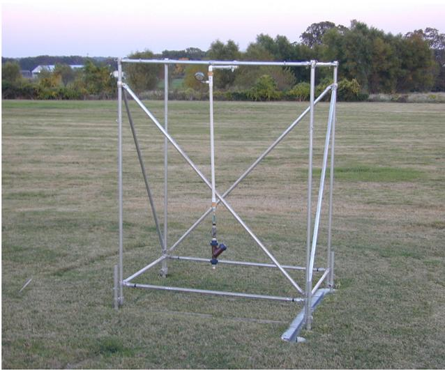
Figure 1. Portable rainfall simulator shown over 1.5- × 2.0-m plot.
