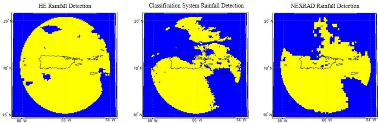
Figure 3. Rainfall detection comparison between the HE (left), the cloud classification system (center), and NEXRAD (right) for October 28, 2007 at 1815 UTC.
