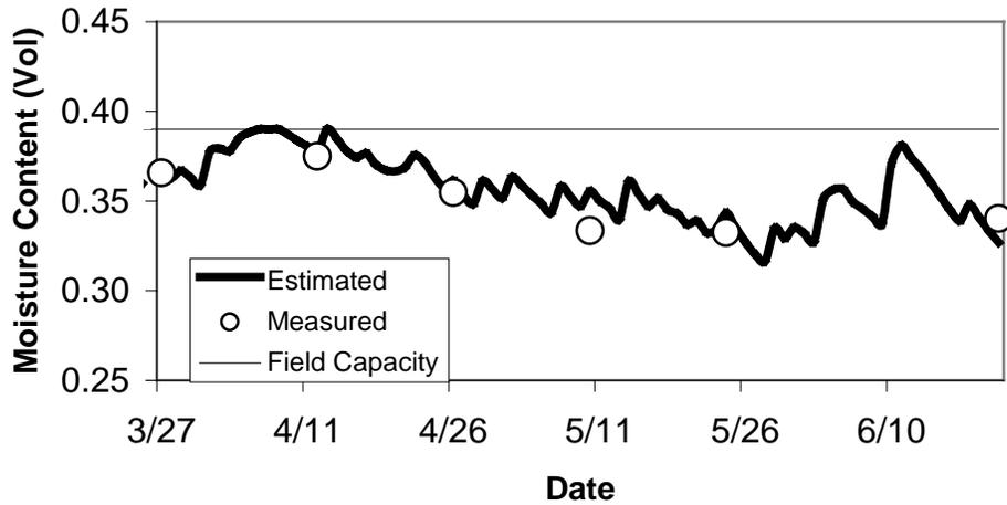
Figure 3. Estimated and measured volumetric soil moisture content.
