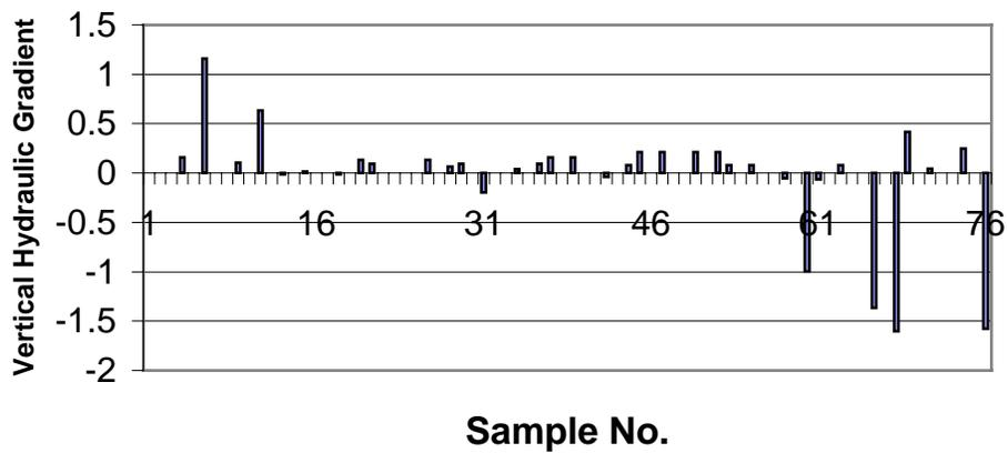
Figure 5. Vertical hydraulic gradients between approximately 50 and 80 cm depths. A positive value represents a downward gradient. Soil pressures were measured using tensiometers.
